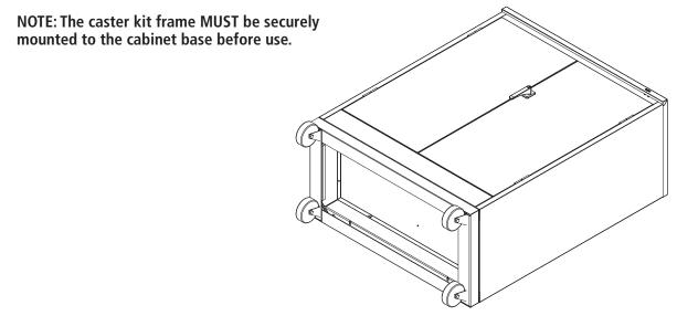
**8.** Carefully set the unit upright on its casters. To prevent the unit from rolling during this process, two people are recommended to preform this step. The cabinet is now ready for mobile use.
