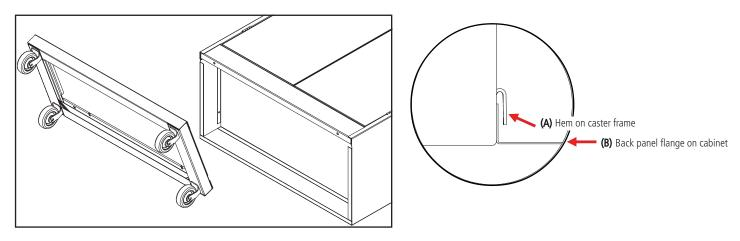
**6.** Secure the cabinet to the caster kit frame by attaching at the front with two  $5/16'' - 18 \times 3/4''$  bolts and nuts (Ref. Nos. 4 and 5) through the sill. Use a 1/2'' wrench to tighten securely.
