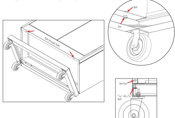
7. Before setting the storage cabinet upright, be sure that all bolts and nuts are tight and that the frame is secure.
